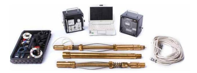
This system was built to control HDD process with big depth and length. Working principle is based on measuring of gravity and magnetic field of the Earth using special sensors in the probe. All data goes by cable to the Interface module of the system for decoding. From module data goes to PC where it is calculating to define depth, probe position, angle etc. Final information is assembling to convinient table and goes to Control Panel of Drillmaster.
