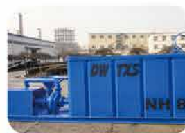
Mud mixing unit
